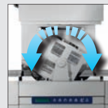
Caps crate rotation forward - backward during the wash phase
