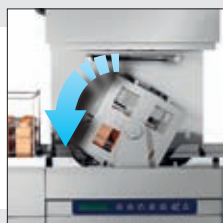
Rotation for bottle emptying, washing and rinsing
