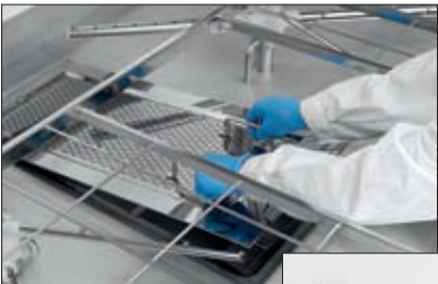
Self-cleaning filter for recirculation of the washing water.
